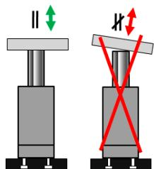
The nitrogen cylinder must be installed at a right angle to the acting force.
