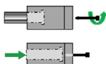
Prior to dispatch, used nitrogen cylinders must be emptied with the designated discharging screw. When emptying, point the filling opening away from the operator. To make sure that the nitrogen cylinder is fully decompressed, completely push the piston in by hand.
