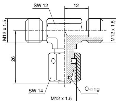
**T-coupling with sealing taper**
