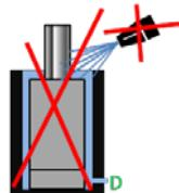
Protect the piston rod from contact with liquids.
