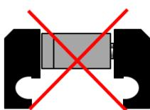
For clamping of the nitrogen cylinder, always use an appropriate fixture (jaw chuck, vise jaw with tread).
