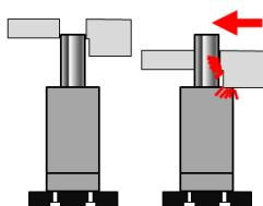
It is important to make sure that the nitrogen cylinder in the tool does not touch movable parts.
