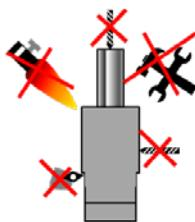
Nitrogen cylinders with signs of damage may not be used.
