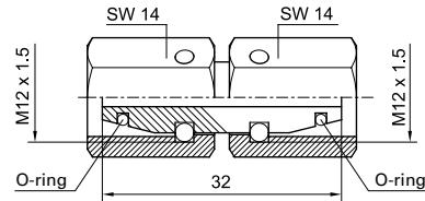
**Straight intermediate connection piece with sealing taper**
