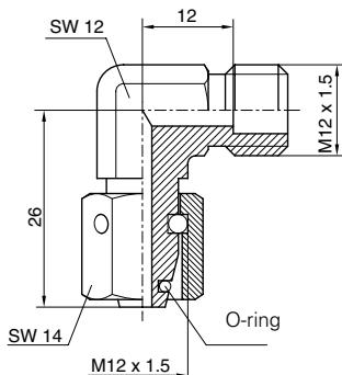
**Elbow connection with sealing taper**
