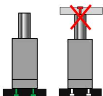
The nitrogen cylinder must be screwed on at the base and never at the piston. Screws with the strength class 8.8 are recommended for tightening. The tightening torques are to be selected according to VDI 2230.
