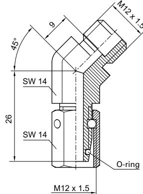
**45° elbow connection with sealing taper**
