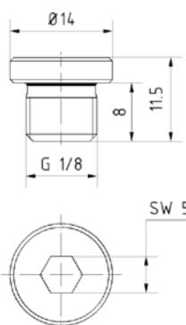
**Sealing plug with seal**
