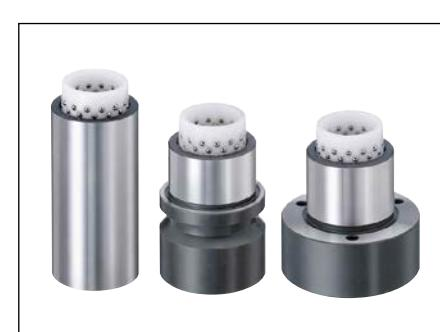
**Plastic ball cages** are particularly distinguished from other materials by the lower weight. They are used wherever there are high stroke frequencies. In addition, the plastic is suitable for aggressive ambient influences.
