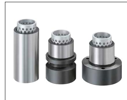
**Aluminium ball cages** are distinguished from the brass by the significantly lower weight. Due to the cage's mere carrier function, each reduction in weight (with the same level of stability) means smaller inertial forces, especially in the movement turning points.
