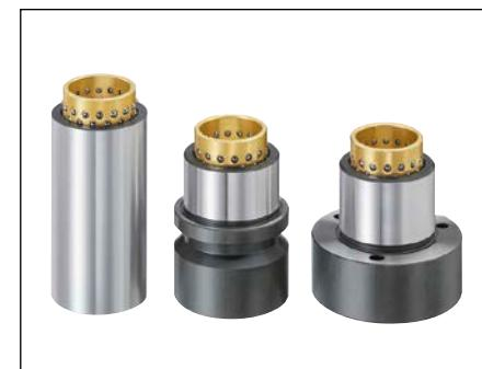
**Brass ball cages** are universally suitable. They have a high mechanical strength and the best sliding characteristics, as well as high wear resistance and stability. Due to their optimal thermal stability, they are suitable for temperatures above 80 °C/176 °F. Very robust versions, suitable for machines and tools with high accuracy requirements.
